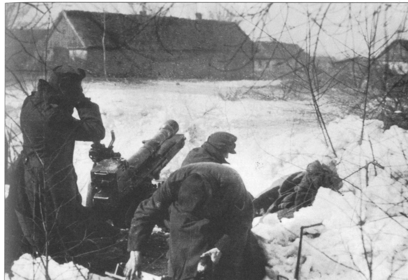
During a defensive action a 7.5cm Geb36 gun crew can be seen with their weapon. Firing an artillery piece in the snow could be frequently problematic for the gun crew. The recoil would regularly drive the weapon deep into the snow and would often cause inaccurate firing. For this reason this 7.5cm Geb36 gun has been modified – its wheels have been removed and replaced with sturdy gun trails
