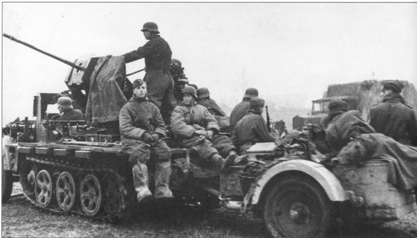
Grenadiers are hitching a lift onboard a Sd.Kfz.10/4 halftrack. The vehicle mounts a 2cm Flak 30 gun. Note some of the troops on the Sd.Ah.51 trailer. The Flak30 was used extensively on the Eastern Front and had a maximum rate fire of 120 rounds per minute, with a horizontal range of 4800 metres.
