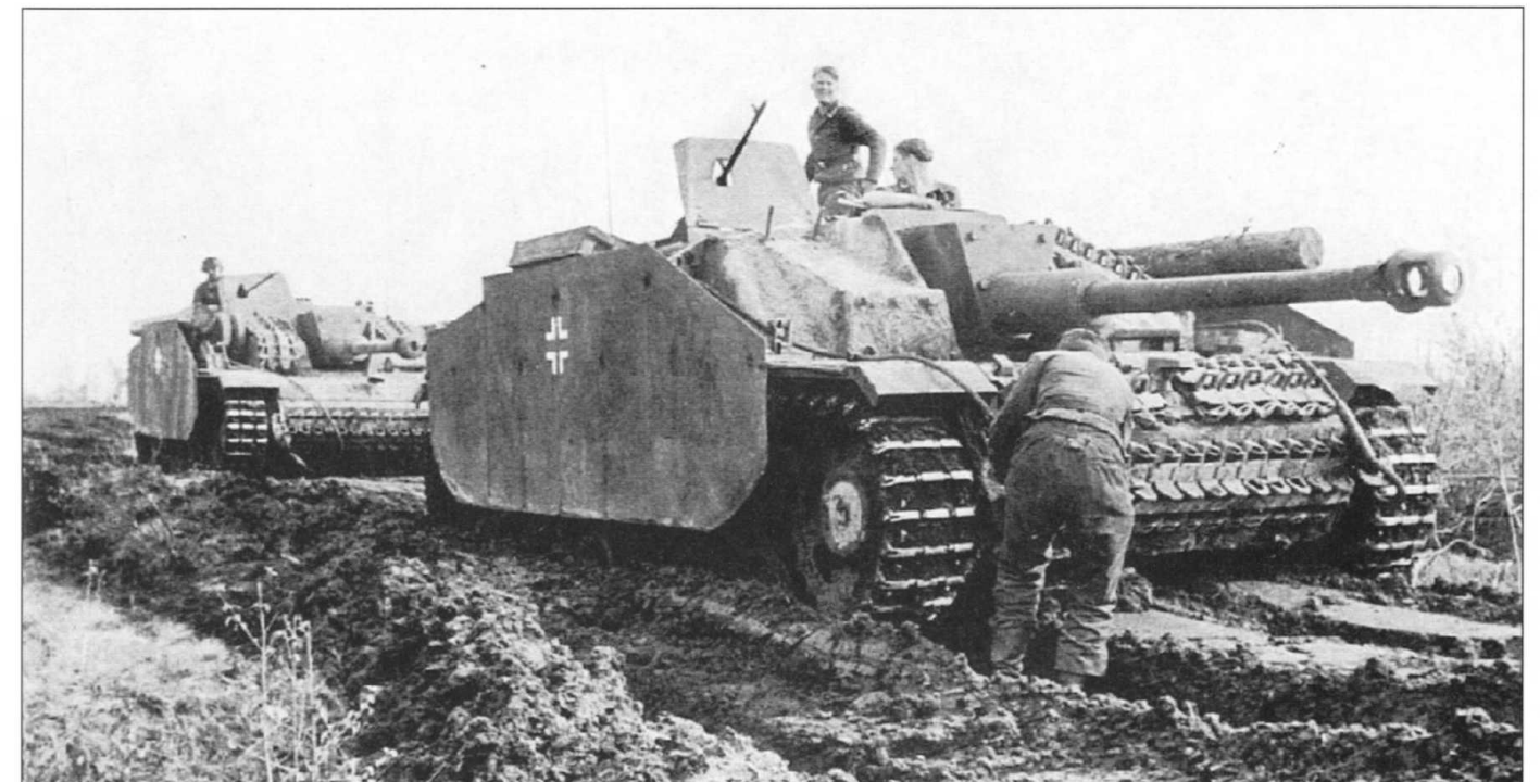
Two StuG.III Ausf.Gs along a muddy road in Latvia after a heavy downpour of rain. The leading StuG appears to be getting some assistance as it's stuck in the mud. Note the track links attached to both vehicles for additional armoured protection. Both the StuGs are armed with an MG34 machine gun with a folding cast armoured shield, which was used to protect the gunner against aerial attack.
