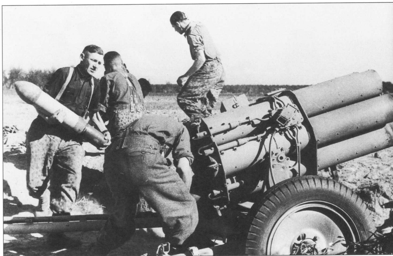
A Nebelwerfer crew is loading the rocket shells into the Nebelwerfer 41. The Nebelwerfer 41 was equipped with six barrels, each firing a 34 kg (75 lb.) 150 mm (5.9 in.) Wurfgrate 41 (rocket shell 41) rocket out to a range of approximately 6800 meters (7437 yards). Along the Narva front the Nebelwerfer was used extensively and caused high losses in the Russian lines.
