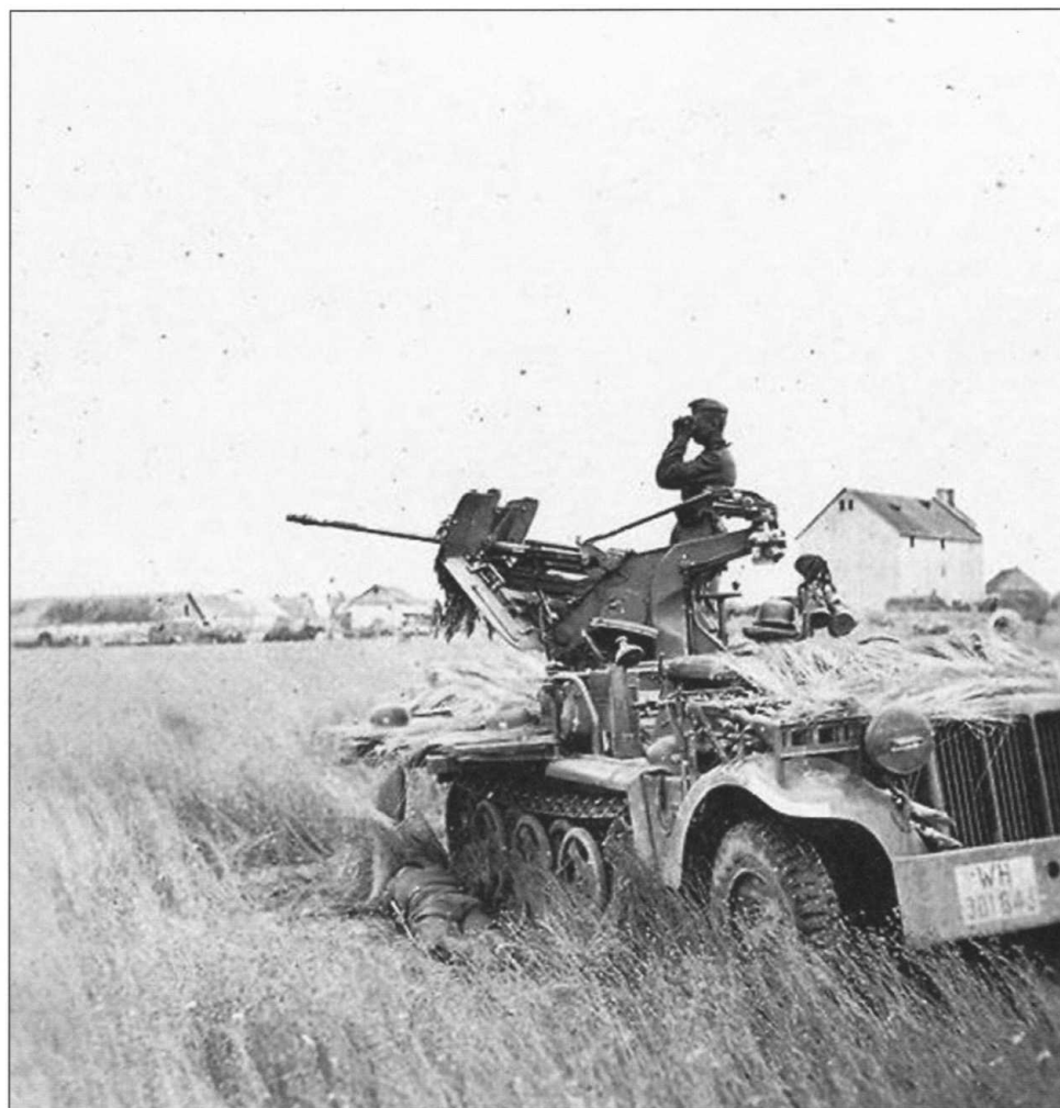
A 2cm Flak gun mounted on the back of a half-track in a field with one of the crew members scouring the terrain for enemy activity. The sides of the vehicle are folded down. The sides allowed extra space on board the halftrack for the flak crew to easily manoeuvre.
