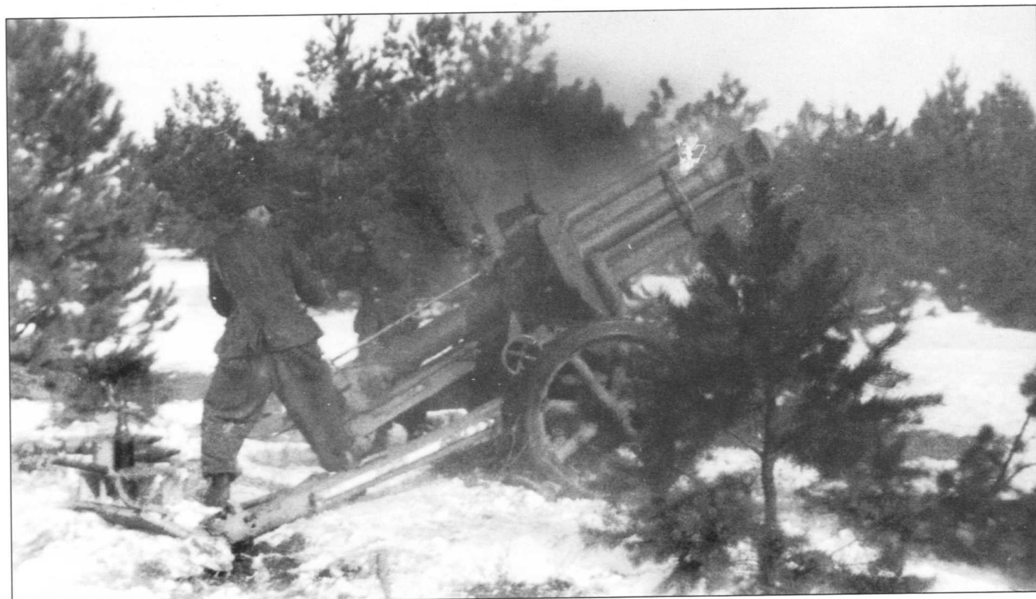
A photograph taken the moment a 10.5cm I.FH18M gun's projectile leaves the barrel during defensive action in early 1944. These light field howitzers were constantly modified during the war in order to increase their ranges. Even as the Germans steadily withdrew combat experience soon showed that artillery support was of decisive importance in both defensive and offensive roles.
