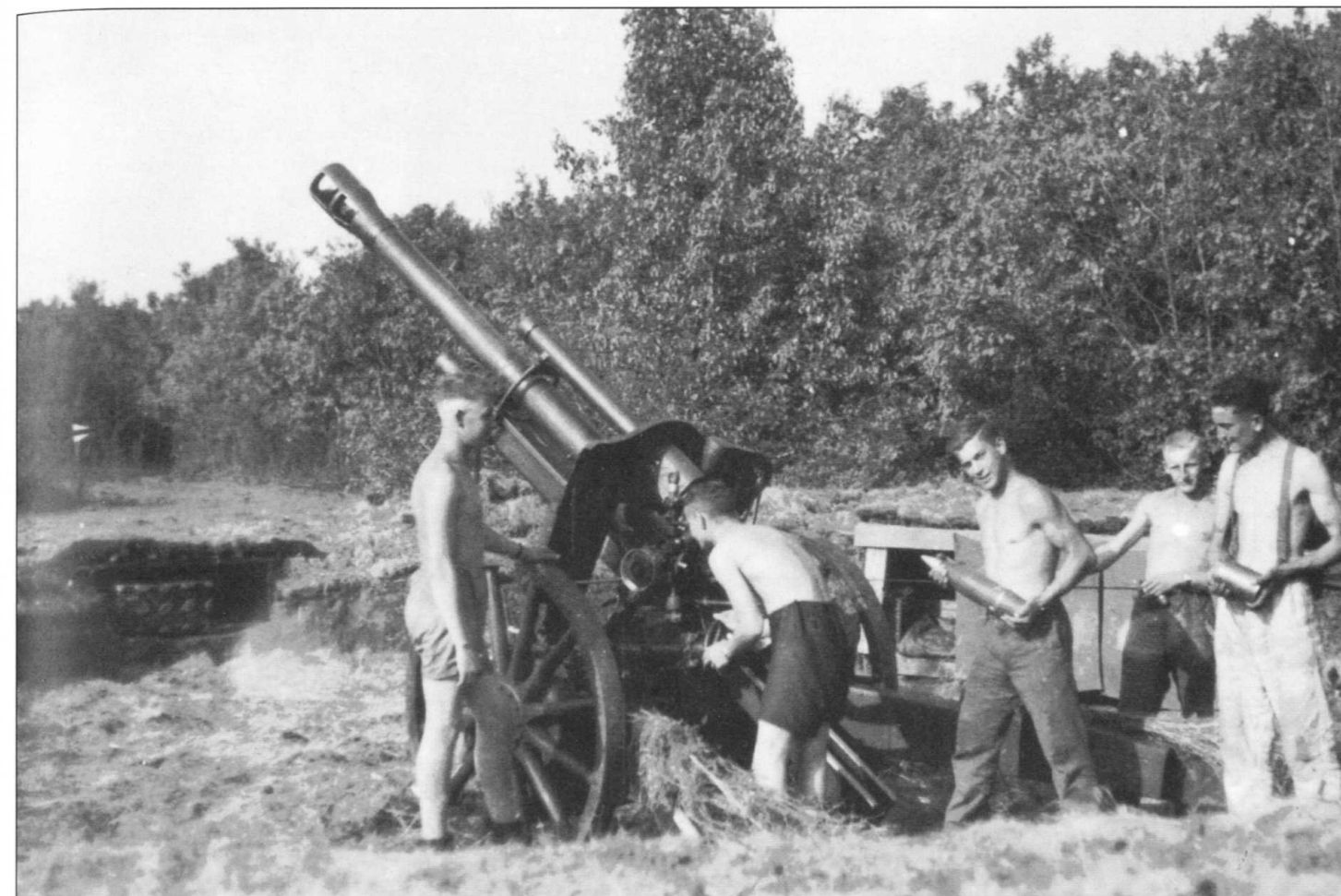
Two photographs showing gun crews preparing to fire modified 10.5cm le FH 18/42 guns in anger. The 10.5cm was the standard light artillery piece deployed in the artillery divisions on the Eastern Front. However, in order to give the gun better punch on the battlefield the weapon was modified in 1942. The barrel was lengthened, a cage muzzle-brake was fitted, and the carriage was a lightened version of the le FH 18 design.
