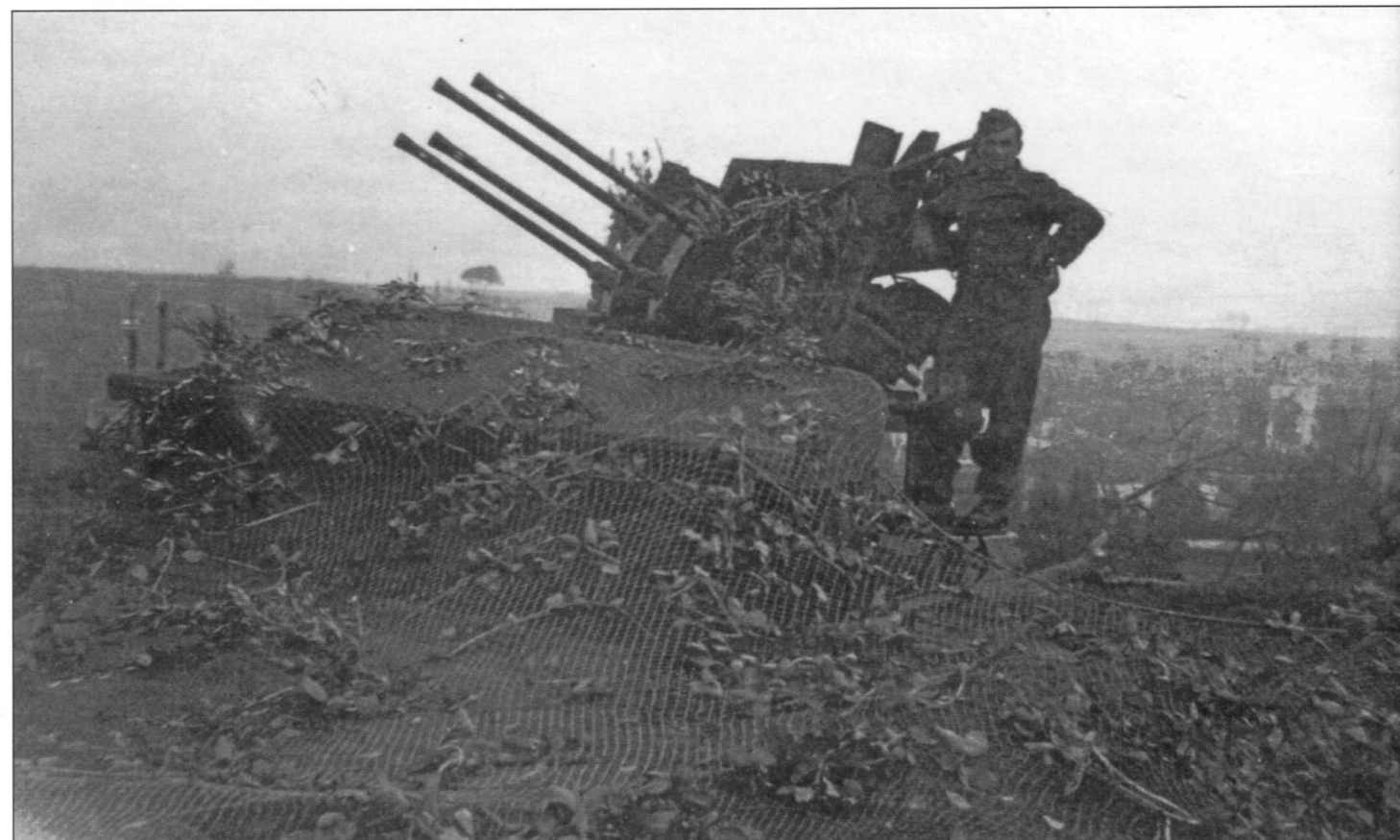
A soldier stands next to a 2cm quadruple self-propelled flak gun during operations in the summer of 1944. This weapon could engage not only air targets but ground ones as well. The gun is in a defensive position and great lengths by the flak crew have gone into camouflaging the position. Note the camouflaging netting with foliage draped over the crew's shelter.
