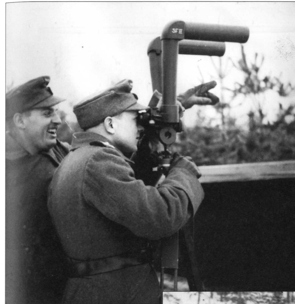
In a forward observation post a soldier can be seen peering through a 6x30 Sf.14Z scissor periscope to search for, detect, plot, and determine the direction to targets. Along huge parts of the front in Army Group North the lines were relatively stagnated sometimes for many weeks. Troops were constantly surveying the front in order to keep a daily check on the location and movement of their enemy.
